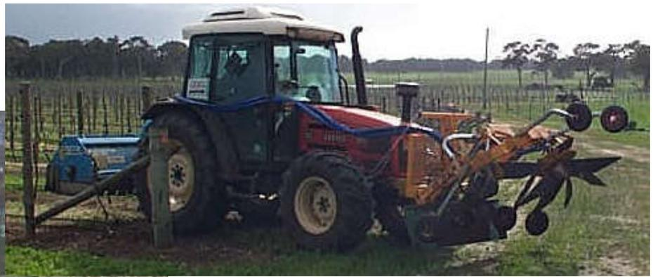
This SADIE is mounted onto the tractor's front bumper bar (not included). The bumper bar is supplied (100x50x6 RHS steel tube) but without brackets as these need to be made to suit the tractor and welded to the RHS. The SADIE clips over this and is held on with bolts. There is a tension chain with bracket to be mid-mounted each side (supplied).
