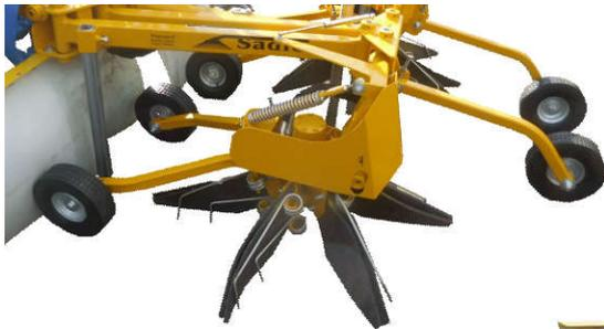
SADIE's Ø8mm spring tynes are bolted in front of the rubber flaps and are adjustable in height. This allows the tyne to be lower than the rubber flap to allow vigorous raking. The tynes are not as long as the rubber flaps to prevent any damage to the vine trunk. You can use with or without tynes to achieve the best results.
