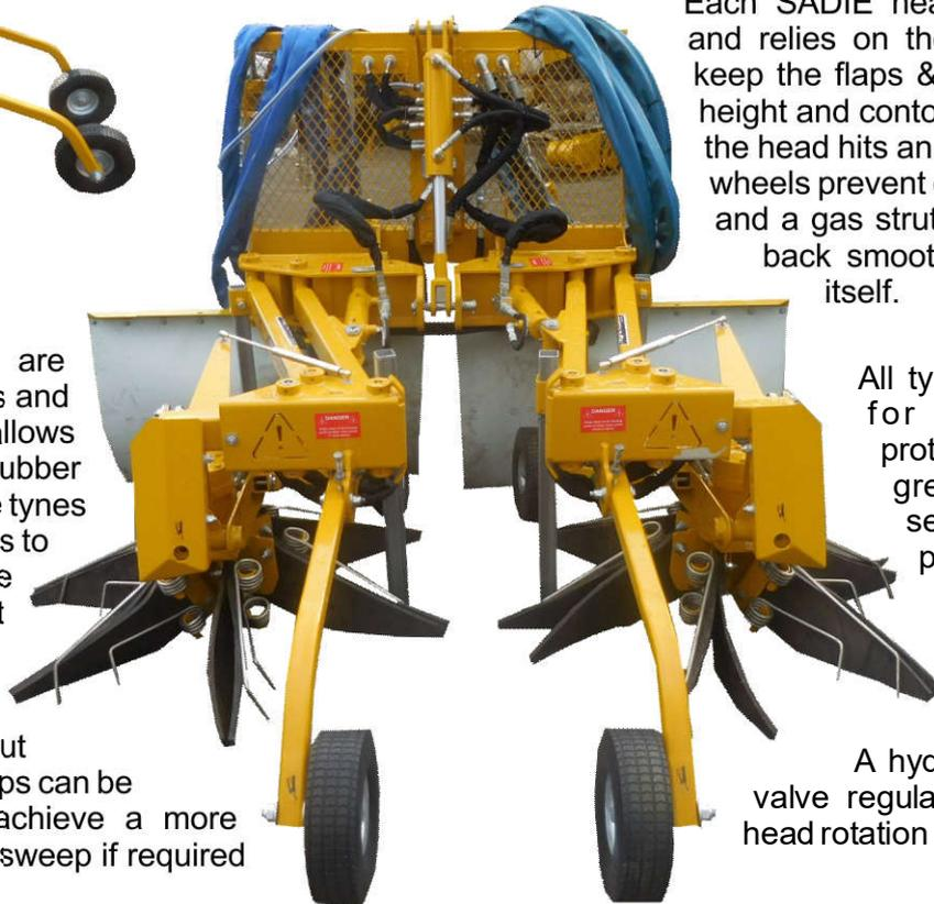
Each SADIE head is independent and relies on the three wheels to keep the flaps & tynes at the right height and contour of the ground. If the head hits an obstacle the guide wheels prevent damage to the vine and a gas strut allows it to swing back smoothly and reposition itself.
