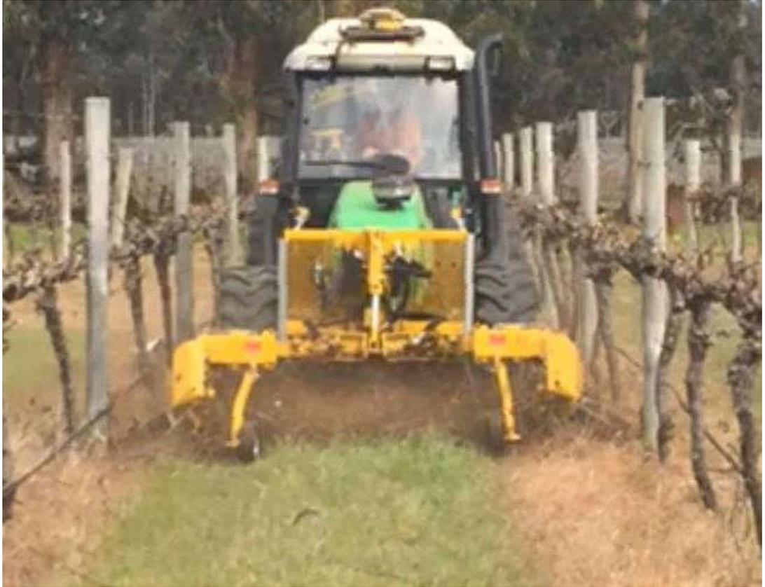
Width setting from 2.2m to 4m is achieved by two synchronised hydraulic rams. Another hydraulic ram raises the heads in any width setting.
